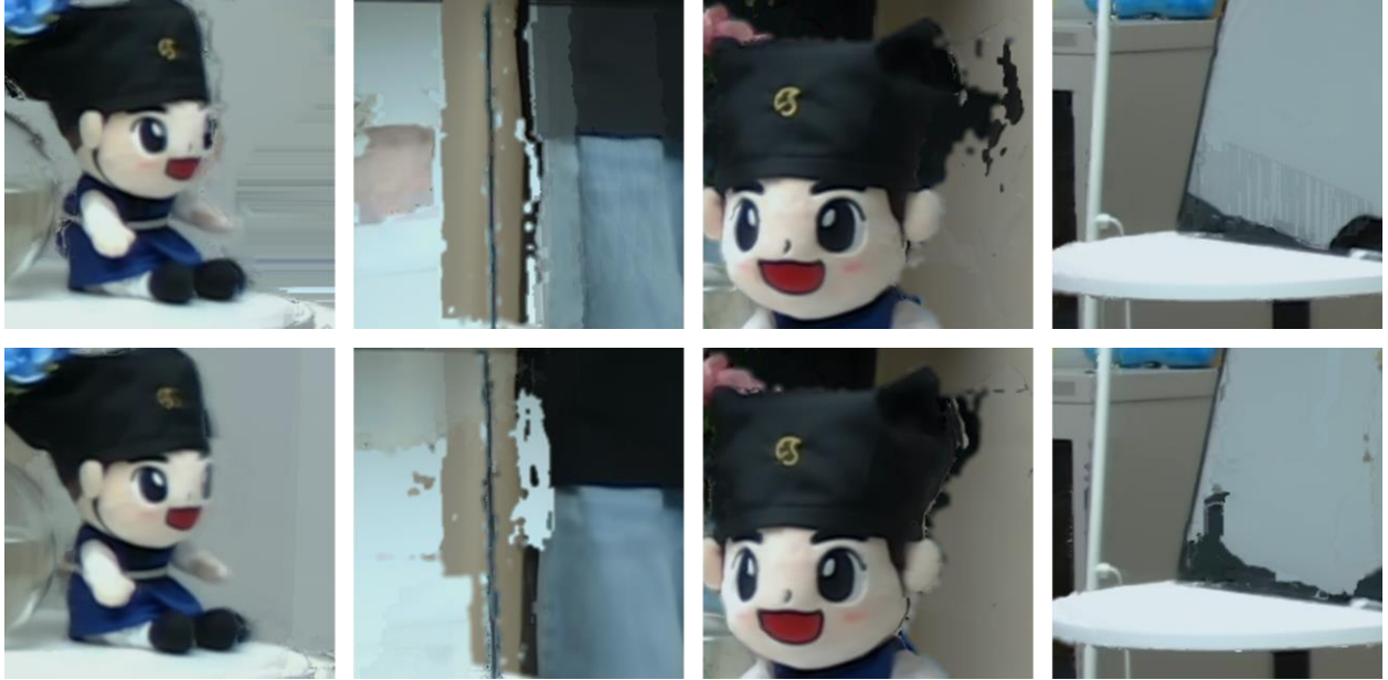
Figure 4. Synthesized test views of source, Partial and Full conditions, first row represents source, second row represents Partial (RP2, 12.26Mbps), third row represents Full (RP2, 12.26Mbps). First and second columns represent v07, third and fourth columns represent v24.
