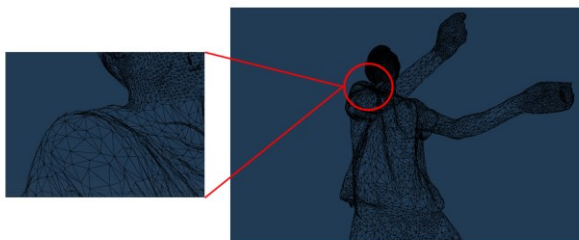
Fig. 1: Structure of a triangulation mesh.
