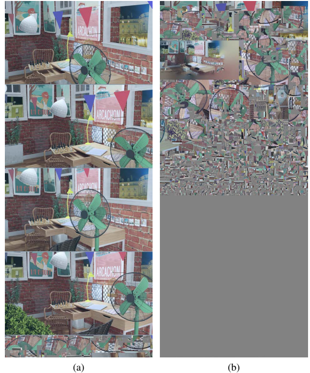
Fig. 1: Examples of texture atlases generated by the MIV encoder: sequence Fan [9], (a) atlas index 0 that mainly contains basic views, (b) atlas index 1 that contains patches from additional views.
